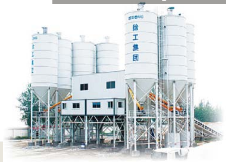
Concrete Mixing Station
