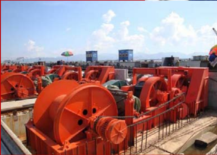
40t friction winch in mechanized comb-type slide control system
